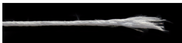
Line failure at approx. 350 daN
